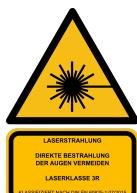
This sensor works with invisible laser radiation of 850nm wavelength! Only operate the sensor with suitable protective equipment against the emerging laser radiation. Never look directly into the laser outlet opening, as long as the sensor is connected!
